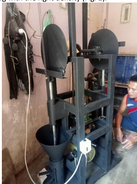
Figure 2. Two-lever baglog press machine
