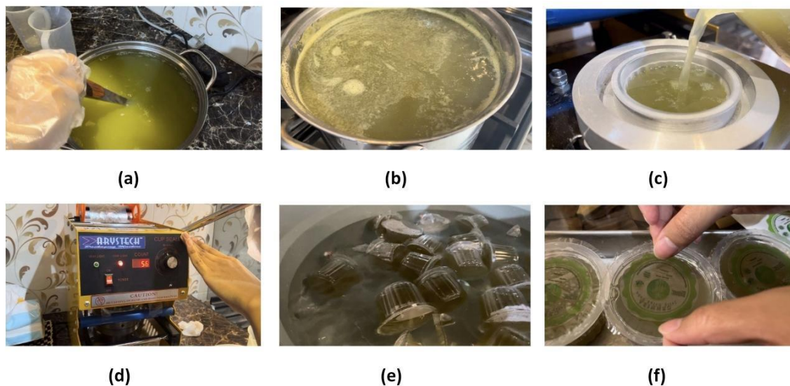
Figure 1. Production Process of Sari Tebu Ijo Jelly Drink. a) Mixing; b) Cooking; c) Pouring; d) Packaging; e) Cooling; f) Labeling.
