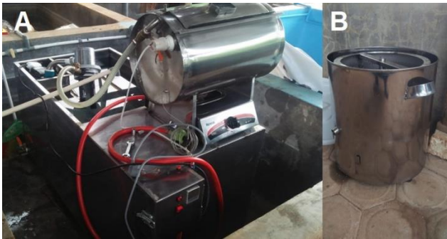
Fig. 1. Relief Tool for Healthy Catfish SME (IGF). A: Vacuum frying and B: spinner
