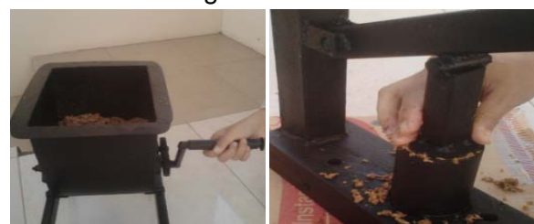
Figure 1a. Kneading machine sawdust briquettes and starch, b. Press tool sawdust into briquettes.
