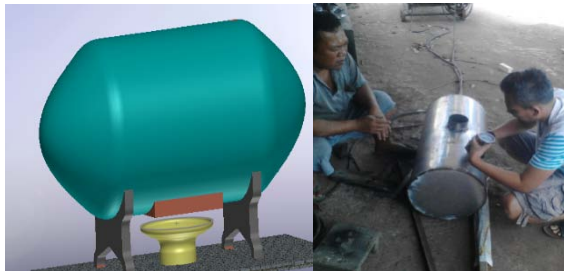
Figure 2. a. 3D design of tool pasteurization, b. Coordination the manufacture pasteurization tube fueled sawdust wood briquettes.
